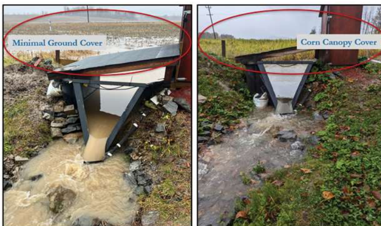
The same surface runoff monitoring location at the corner of the previously untilled field is pictured at different times of the year. Notice that despite the same approximate rate of drainage, the potential for increased erosion when there isn't a growing crop to anchor the soil in place and protect the soil from raindrops with its leafy canopy.
